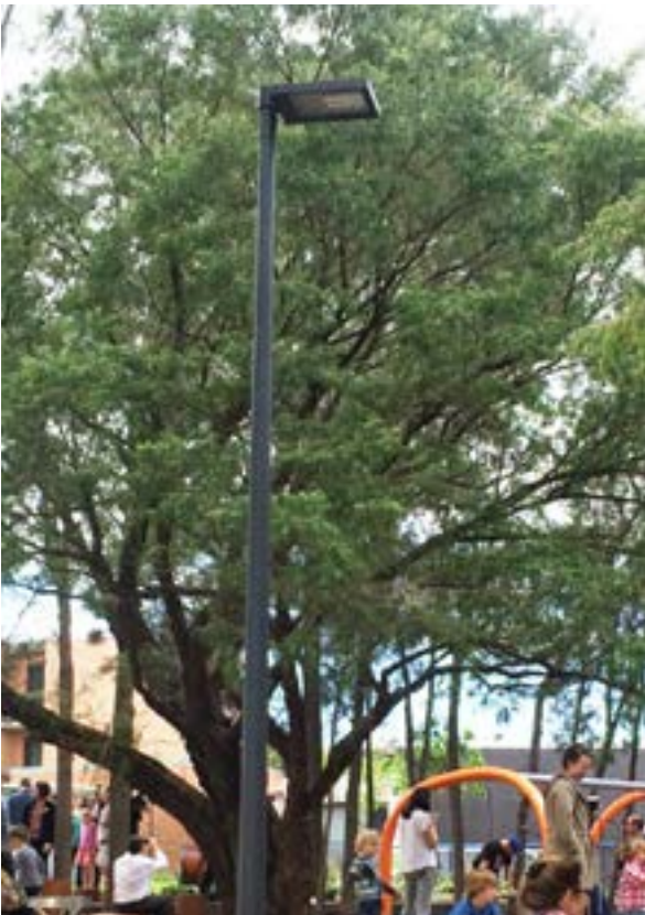
② Laneway lighting to match 105 Phillip St lane. WE-EF VFL520 LED (700mA) 108-1502. (or equal)
